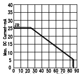
Fig5. MAX. ALLOWABLE DC CURRENT VS. AMBIENT TEMPERATURE.
