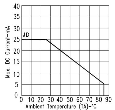
Fig5. MAX. ALLOWABLE DC CURRENT
