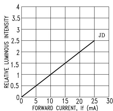
Fig3. Relative Luminous Intensity
