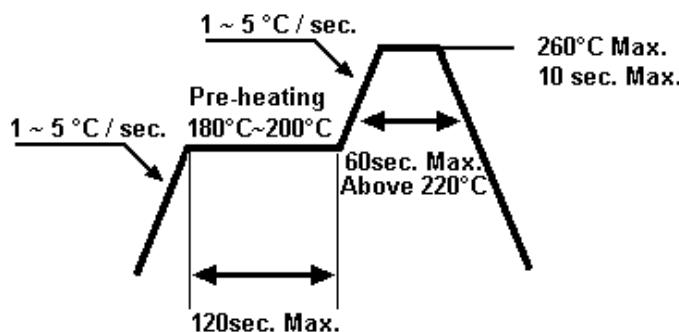
4.2.2 Reflow soldering should not be done more than two times.
