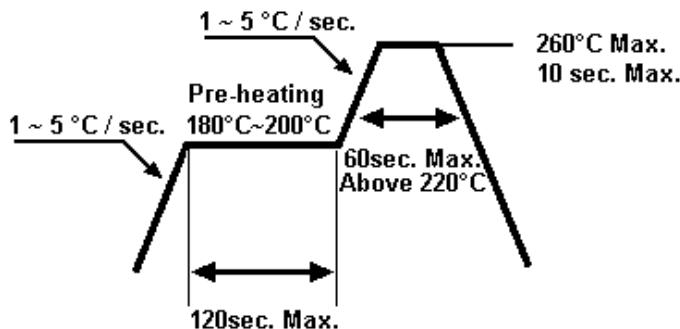
4.2.2 Reflow soldering should not be done more than two times.
