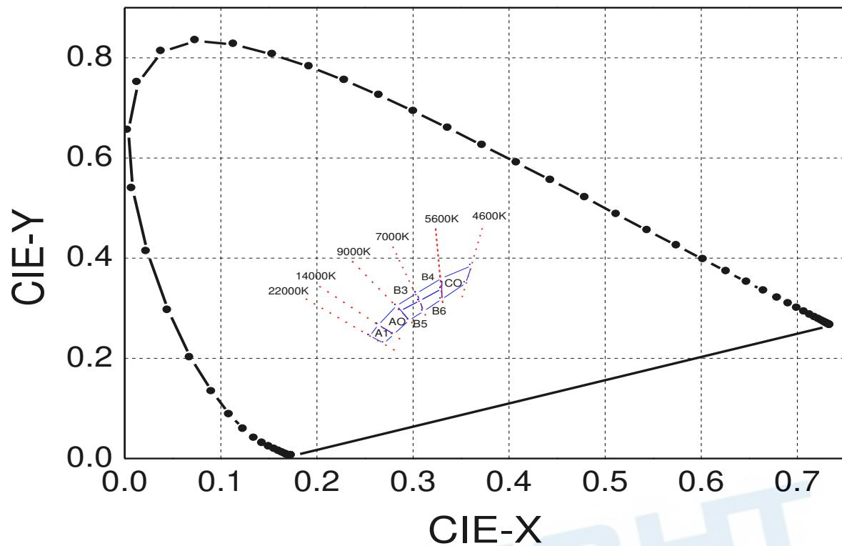
Color Ranks ( $I_F=20\text{mA}$  ,  $T_a=25^\circ\text{C}$ )
