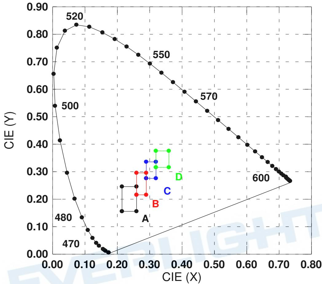
Color Ranks ( $I_F=20\text{mA}$  ,  $T_a=25^\circ\text{C}$ )
