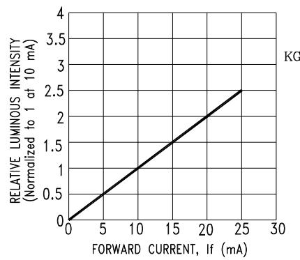
Fig3. Relative Luminous Intensity
