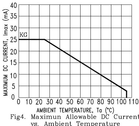
Fig4. Maximum Allowable DC Current
