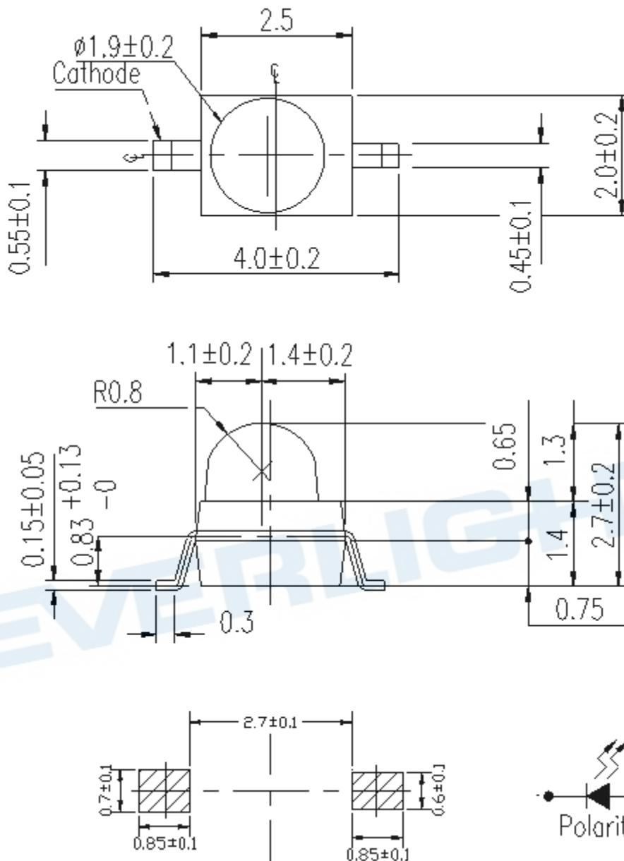
Note: The tolerances unless mentioned are  $\pm 0.1$ , unit=mm.
