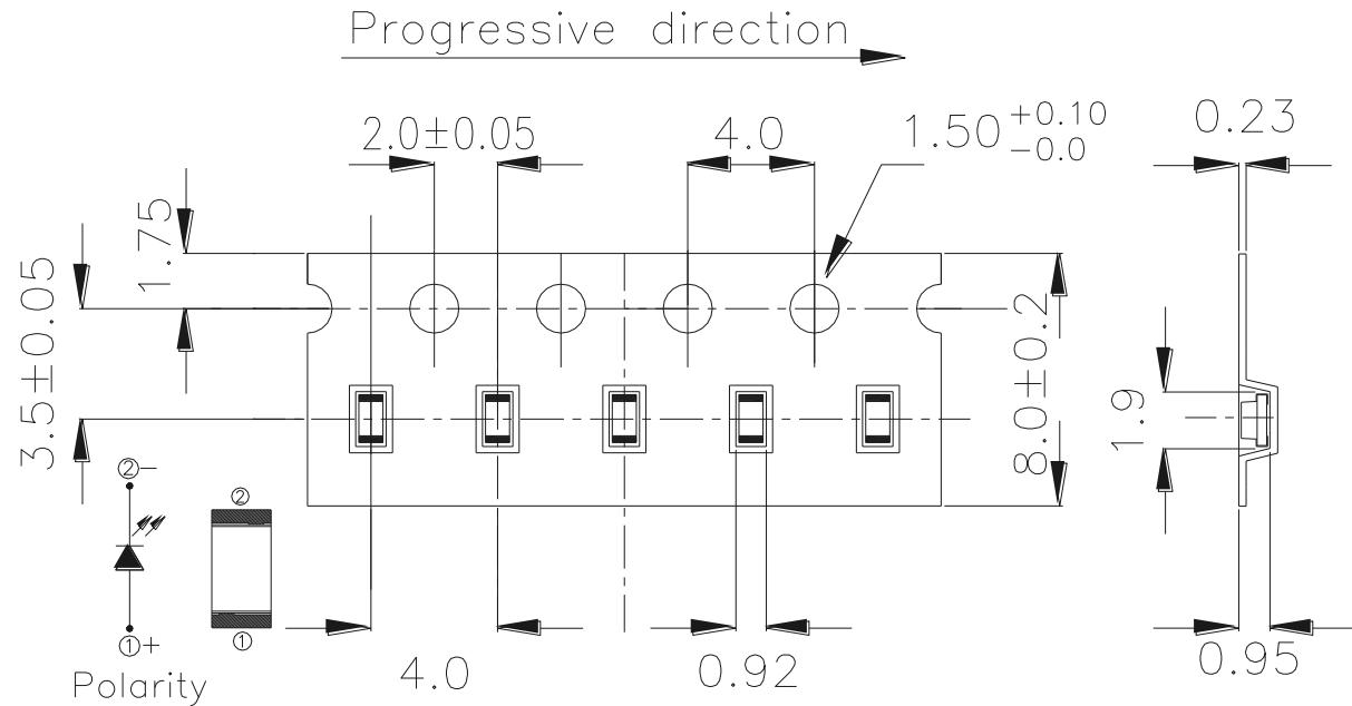
Note: The tolerances unless mentioned is  $\pm 0.1\text{mm}$  ,Unit = mm
