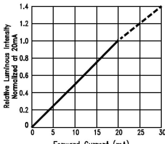
Fig.4 Relative Luminous Intensity
