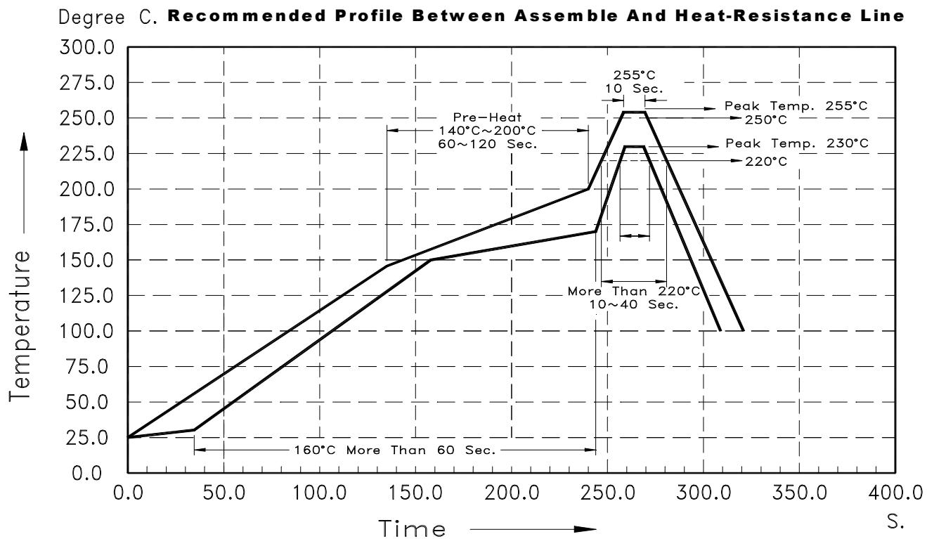
**The Profile is available that must to use SnAg ( $x=3.3\sim 3.8$ ) Cu ( $y=0.2\sim 0.7$ ) solder paste**
