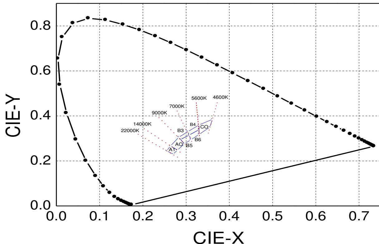
Color Ranks ( $I_F=20\text{mA}$  ,  $T_a=25^\circ\text{C}$ )
